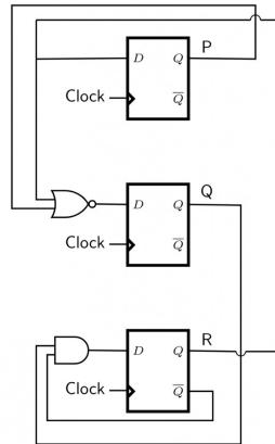
If at some instance prior to the occurrence of the clock edge,  $P, Q$  and  $R$  have a value 0, 1 and 0 respectively, what shall be the value of  $PQR$  after the clock edge?
