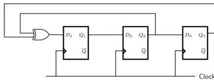
Draw a state diagram, which is implemented by the circuit. Use the following names for the states corresponding to the values of flip-flops as given below.
