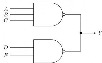
The logic function  $Y$ , implemented by the circuit is,
