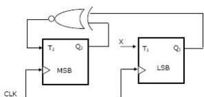
To complete the circuit, the input X should be
