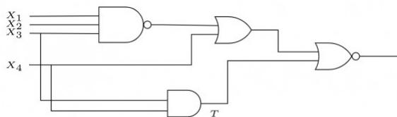
Which of the following inputs ( $X_1X_2X_3X_4$ ) will detect the fault ?
