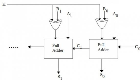
If the operands are in 2's complement representation, which of the following operations can be performed by suitably setting the control lines  $K$  and  $C_0$  only (+ and - denote addition and subtraction respectively)?
