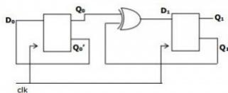
The flip-flops are positive edge triggered D FFs. Each state is designated as a two-bit string  $Q_0Q_1$ . Let the initial state be 00. The state transition sequence is
