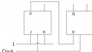
has the initial state of  $P, Q$  as 0, 1 (respectively). After three clock cycles the output state  $P, Q$  is (respectively),
